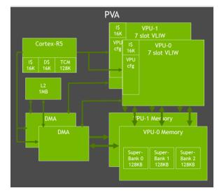
Figure 9: Orin PVA Block Diagram
