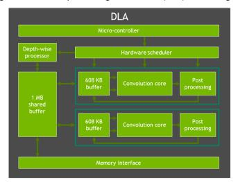
Figure 6: Orin Deep Learning Accelerator (DLA) Block Diagram
