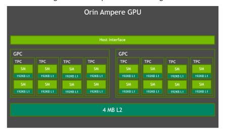
Figure 4: Orin Ampere GPU Block Diagram
