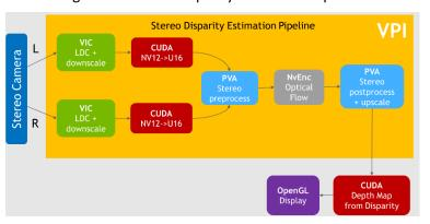
Figure 10: Stereo Disparity Estimation Pipeline
