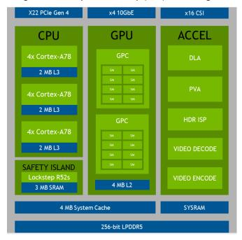
Figure 2: Orin System-on-Chip (SoC) Block Diagram
