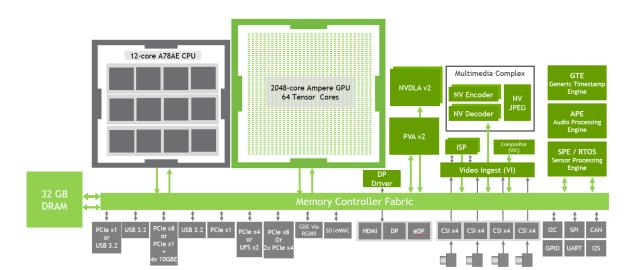
Figure 8: Jetson AGX Orin Functional Block Diagram
