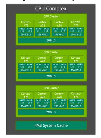
Figure 7: Orin CPU Block Diagram
