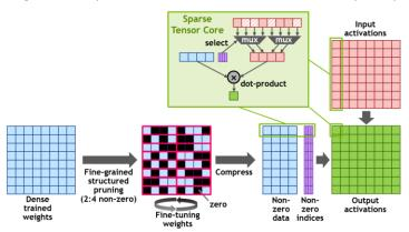
Figure 5: Ampere GPU 3<sup>rd</sup> Generation Tensor Core Sparsity
